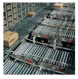
fully Cryovac-wrapped and packed in boxes. Each box contains the same product. The boxes are bar code labeled with the product cut, grade, and net weight, which can be up to 110 pounds. The boxes then travel across a skyway conveyor into the new distribution center, which is kept at a constant 28°F to ensure product freshness. As the boxes move along the skyway, a laser scanner reads the bar code label and updates the inventory. (*Continued*)
